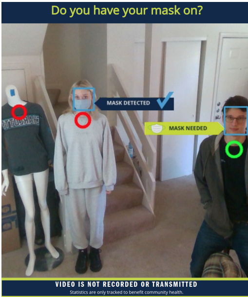
Figure 2: An example of the display while in use (the mannequin is detected as a person by the body pose estimator).
